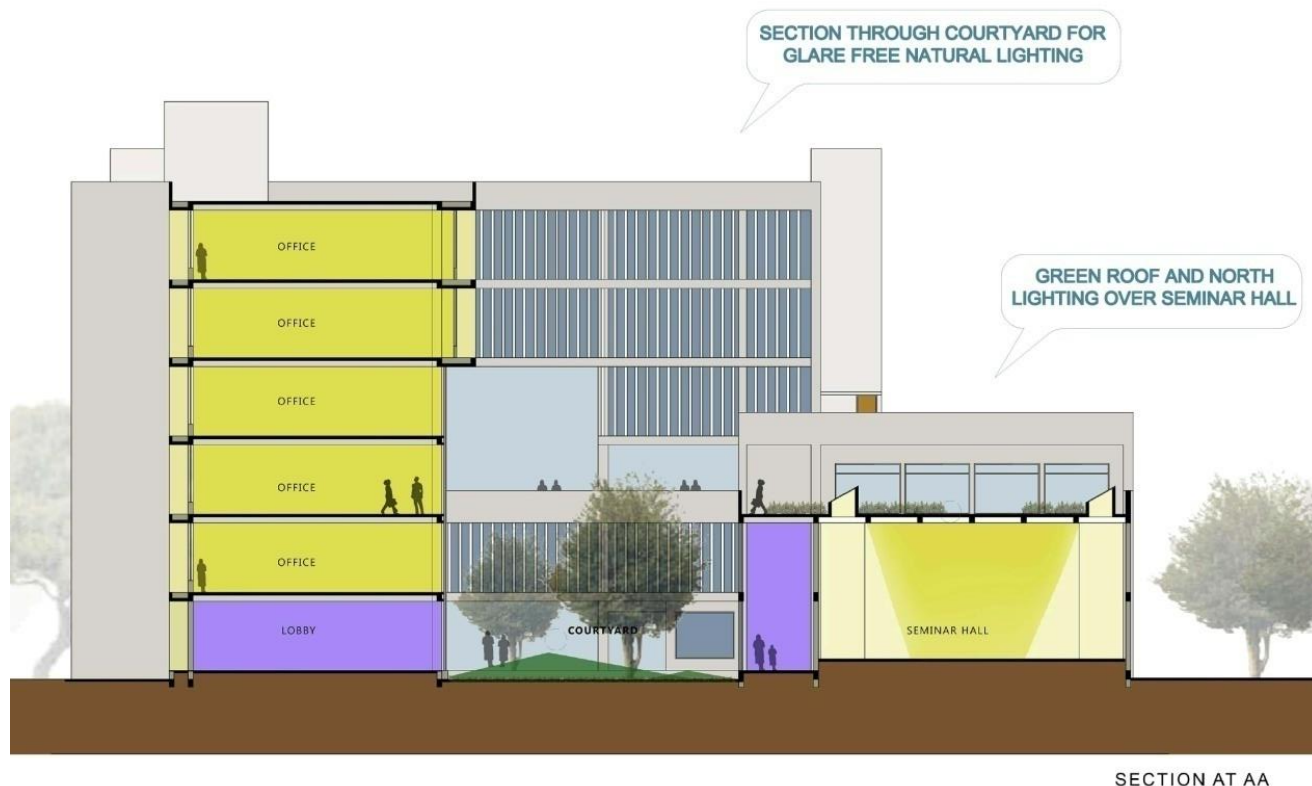
Fig: Section Showing Day Lighting Strategy
