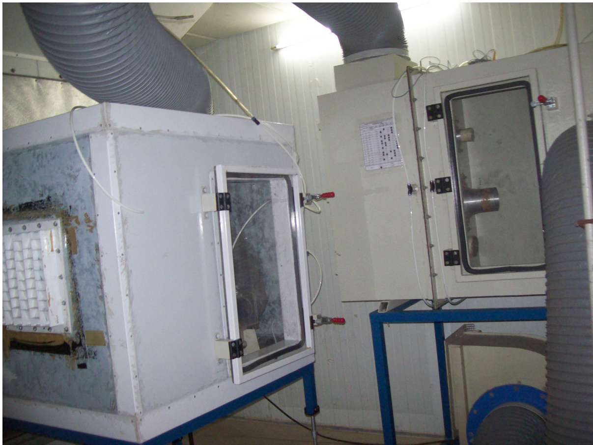
Figure 10: Picture of Code tester: Air flow measurement apparatus
