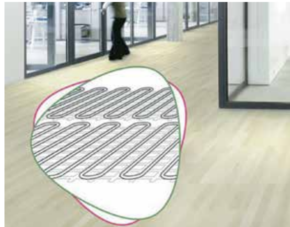
Figure 10: Radiant floor cooling system layout (Rehau.com, 2017)
