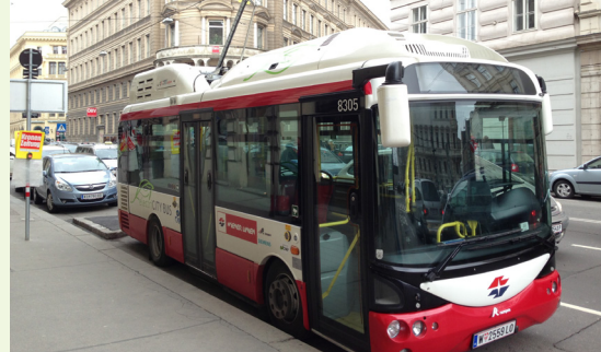
FIGURE 5: ELECTRIC BUS CHARGING VIA CATENARY USING AN ON-BOARD BOTTOM-UP PANTOGRAPH SYSTEM IN VIENNA [SOURCE: (WIKIMEDIA, 2013)]
