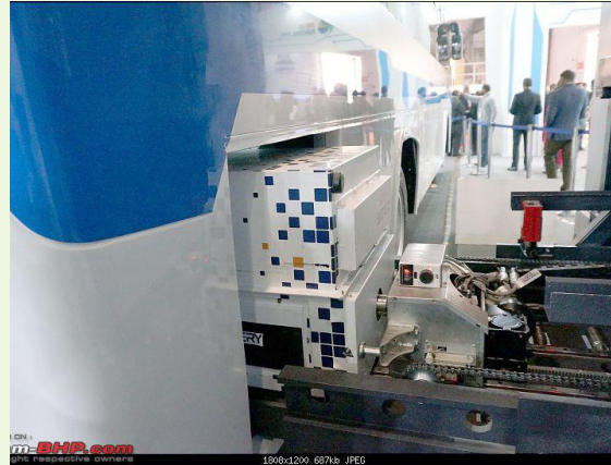
FIGURE 10: BATTERY SWAPPING DEMONSTRATION FOR THE E-BUS MODEL USED IN AHMEDABAD, INDIA [SOURCE: (REHAAN, 2018)]
