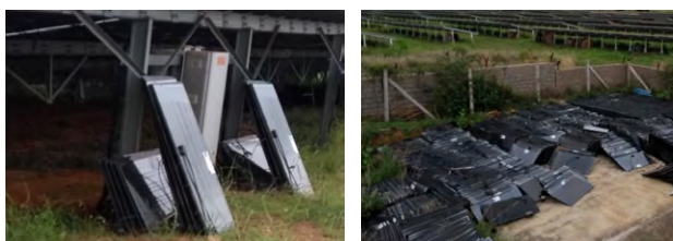
Figure 7: Faulty PV panels in 7 years old utility scale power plant
