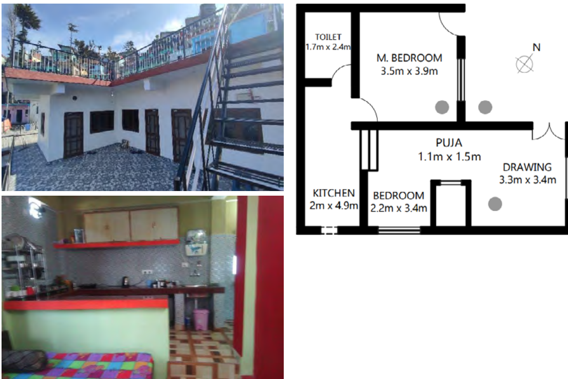
Figure 9-5. Exterior view, interior view, and floor plan showing the sensor location in House C
