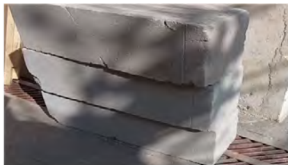
Step 1: 200 mm thick AAC Block
