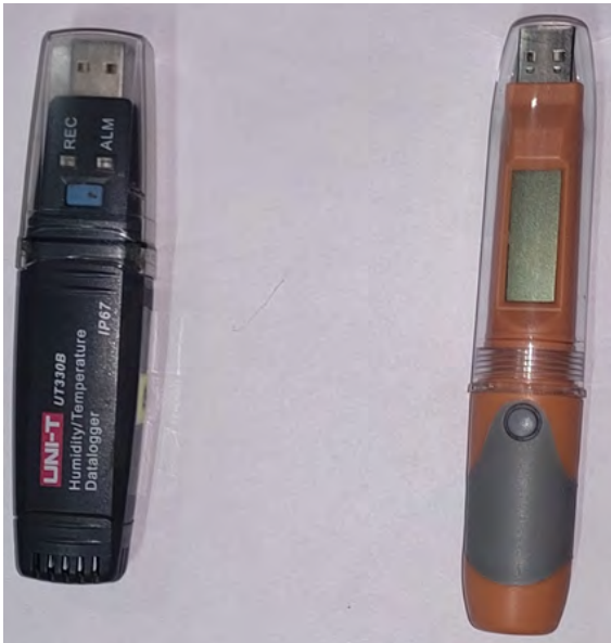
Figure A.1.12. Instrument used to collect indoor and outdoor temperature and humidity
