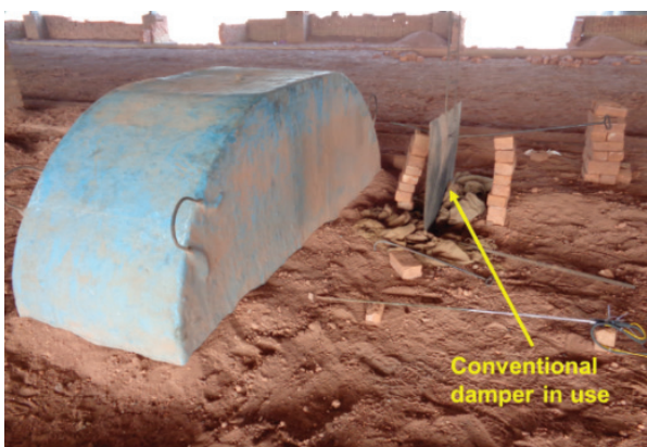
Figure 15: Use of Sheet Metal dampers result in air leakage around the edges of the damper
