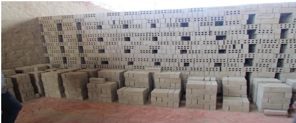
Figure 21: Regular shape bricks and paved leveled floor
