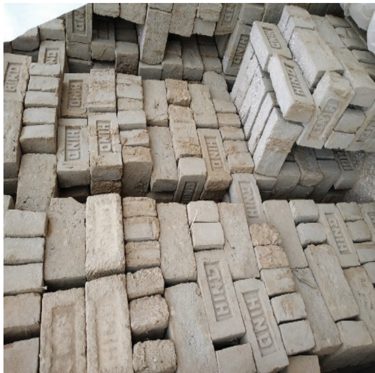
Figure 19 Green bricks damaged by rain being loaded into the kiln
