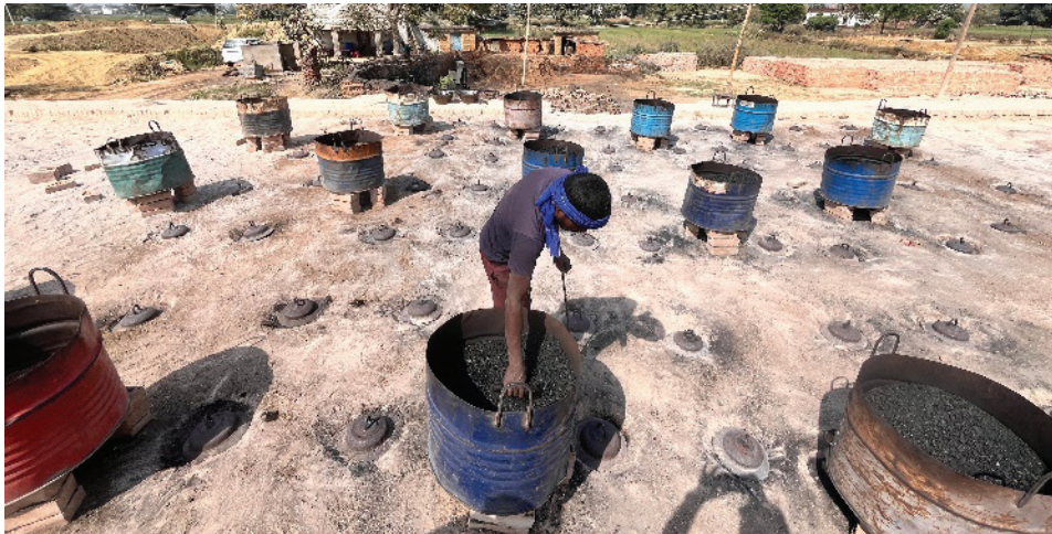
Figure 35 Single fireman continuous fuel feeding.
