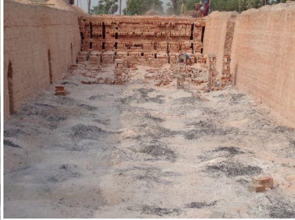
Figure 18: Unburnt coal on the kiln floor
